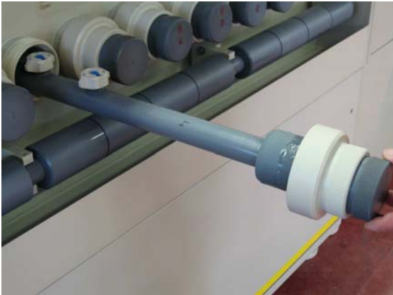
Fig. 3: The transversely installed spray bars can be removed quickly and easily for maintenance work
