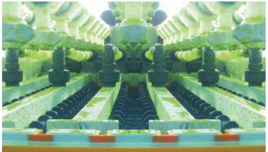
This could be the view into your etching chamber in the very next future: spray bars on top, extraction units between the conveyor rods on bottom
