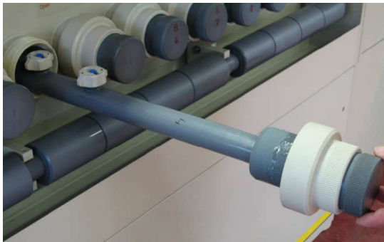
Removed nozzle tube. Vacuum-etching technology
