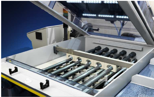
View into an alkaline vacuum-etching modul
