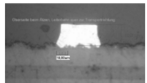
Equal etching results on both the upper and lower surfaces (left), small undercuts and high etch factors after etching (right)
